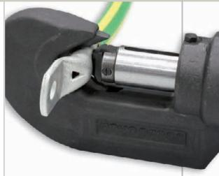
The smart dieless system, developed and patented by Novopress, enables high quality crimps for various makes of cable lugs and sleeves without changing any dies. The HP-Series ensures continual operational readiness, safety and efficiency, on crimps with various cross sections in random order. Compressions will comply with VDE-Standard 0220, NF C 63-061 and SEN 245012.
