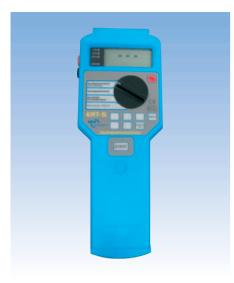
The Earth Resistance Tester is developed for measuring of the earth resistance, possibly with the use of a special current clamp for measuring the soil resistivity on LV-installations according the EN61577 regulation.
